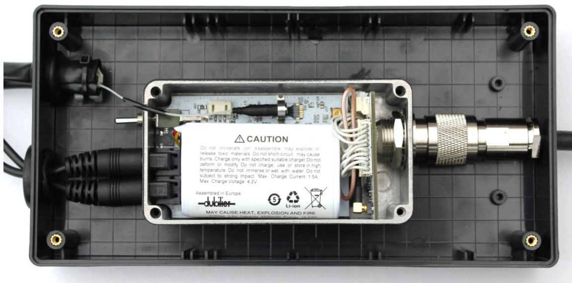
Figure 19 – Sensor head mounted in a plastic enclosure.
